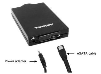
**Step 1:** Connect the eSATA cable to the eSATA port at the back of the enclosure. The other end of the cable connects to the eSATA port on the USB2.0 to eSATA adapter. Plug the adapter to a USB port on your system.
